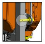
3) Hook up the top three point arm on tractor to the third (top) mounting point on the sprayer and insert the lock pin.
