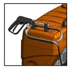
**3)** Remove mounting point pins from accessory box and install on the two sprayer mounting points.
