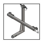
2) Take 3/4" x 4-1/4" quick connecting gold pins and insert into two lower mounting points connecting receiver hitch to unit.
