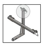
**4)** Next, lift unit using fork points in frame to align receiver mount to hitch.
