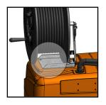
**3)** Tighten the bolts, securely fastening hose reel to tank using a 9/16" wrench.
