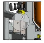
**3)** Then, take 7/8" x 4-1/4" chrome pin and insert in top mounting connection, securing with provided R clip.
