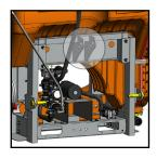
**4)** Route wire harness (make sure wire is not pinched or kinked) to your desired power supply and connect battery cables to their perspective posts. Red to positive post and black to negative post.
