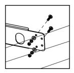
**2)** Slide boom down adjustable brackets, guiding the carriage bolts into the slots.
