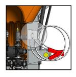
**4)** Adjust regulating valve to aquire desired pressure. Start by threading the regulating valve all the way down (clockwise), then back off 3 revolutions (counterclockwise).
